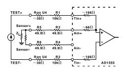
Figure 4. Sensor leakage measurement schematic.
