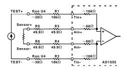
Figure 3. Sensor impedance measurement schematic.
