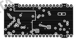
Figure 7. Ground Layer (Not to scale).
