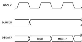
Figure 10. DAC Packed Mode Timing
