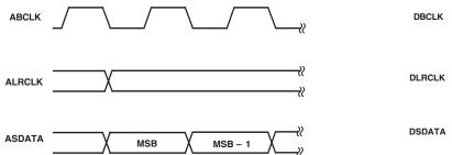
Figure 9. ADC Packed Mode Timing
