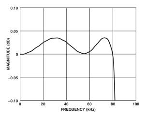
TPC 10. DAC Composite Filter Response,  $f_S = 192 \text{ kHz}$  (Pass-Band Section)
