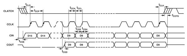
Figure 3. Format of SPI Timing
