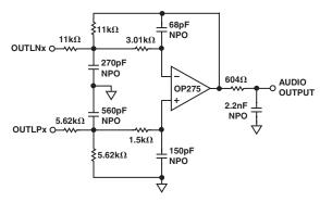
Figure 15. Typical DAC Output Filter Circuit
