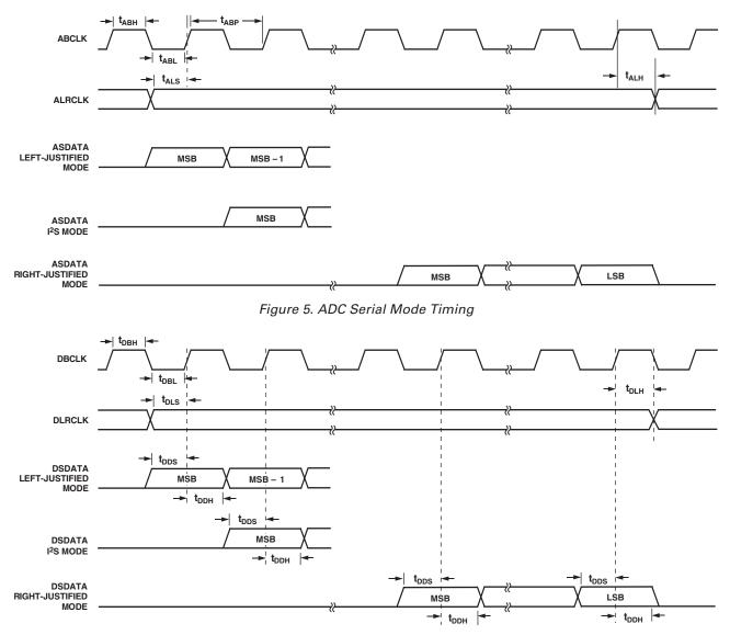
Figure 6. DAC Serial Mode Timing
