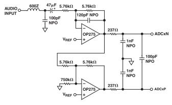
Figure 14. Typical ADC Input Filter Circuit
