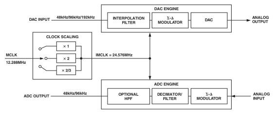
Figure 2. Modulator Clocking Scheme
