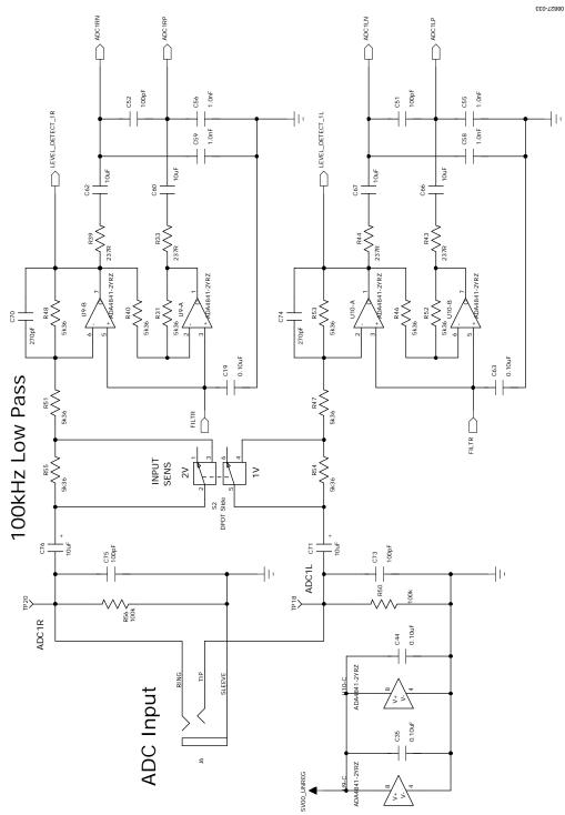
Figure 32. Board Schematics, Page 1—ADC Inputs
