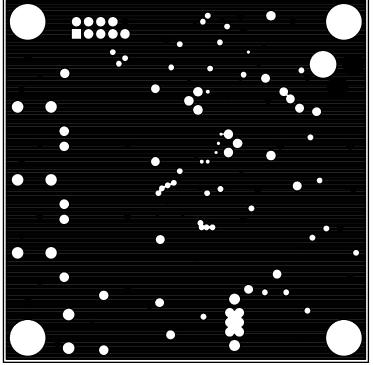
Figure 39. Board Layout, Page 4—Ground Plane
