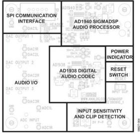
Figure 4. Board Layout Block Diagram (Top Side)
