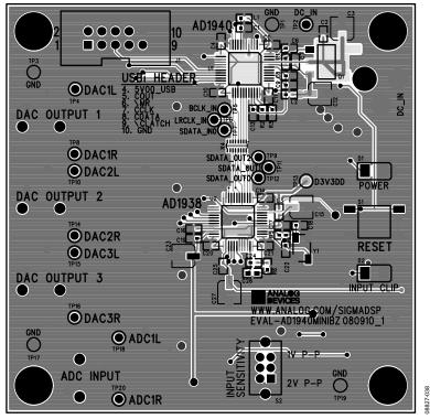
Figure 37. Board Layout, Page 2-Top Layout and Screen
