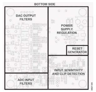
Figure 5. Board Layout Block Diagram (Bottom Side)
