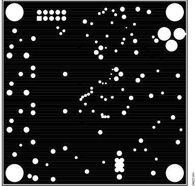
Figure 40. Board Layout, Page 5—Power Plane
