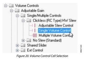
7. Click and drag the **Single Volume Control** cell to the schematic.
