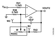
Figure 4. Noninverting Amplifier with Linear Gain
