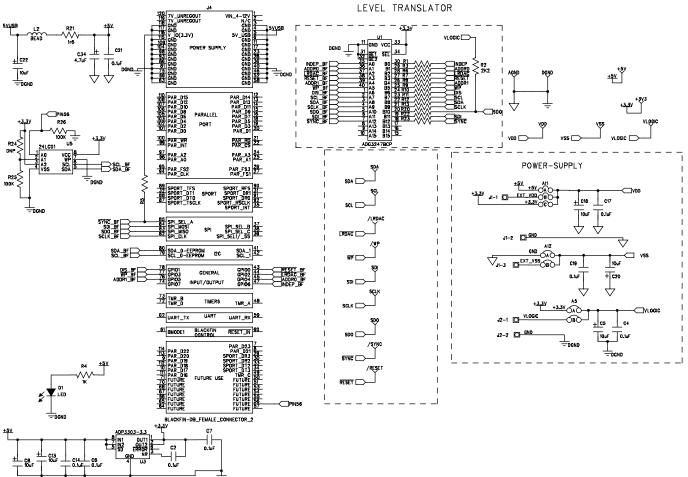
Figure 10. SDP Connector and Power Supply
