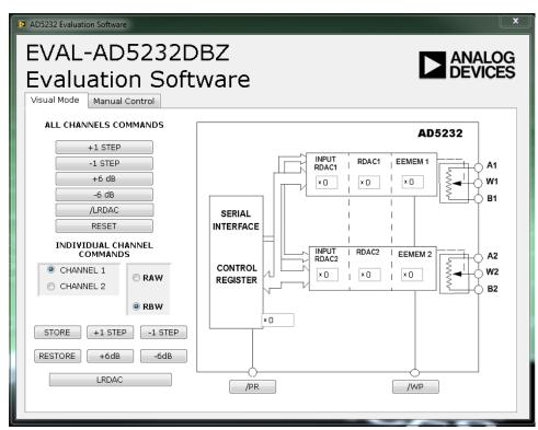
Figure 8. EVAL-AD5232DBZ Software Main Window, Visual Mode Tab
