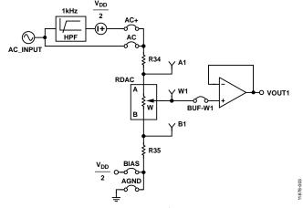
Figure 3. AC Signal Attenuator
