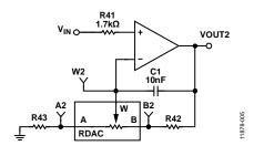
Figure 5. Noninverting Amplifier with Pseudologarithmic Gain
