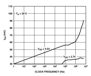
Figure 15. Supply Current vs. Clock Frequency
