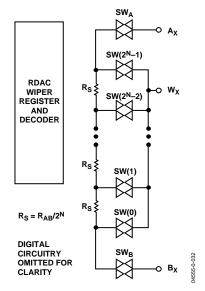
Figure 32. Equivalent RDAC Structure
