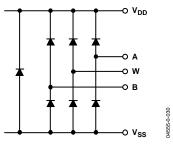
Figure 30. Maximum Terminal Voltages Set by V<sub>DD</sub> and V<sub>SS</sub>
