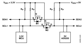
Figure 29. Level Shifting for Different Voltage Devices on an I<sup>2</sup>C Bus
