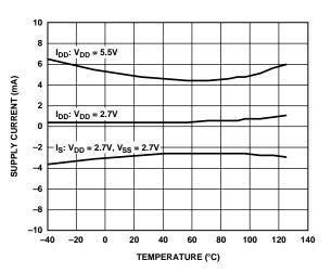
Figure 14. Supply Current vs. Temperature
