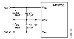
Figure 31. Power Supply Bypassing
