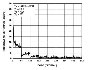
Figure 12. Temperature Coefficient (Rheostat Mode)
