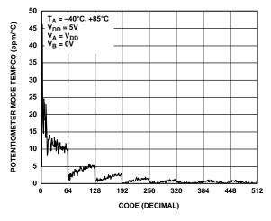
Figure 13. Temperature Coefficient (Potentiometer Mode)
