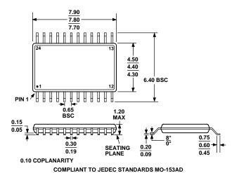
Figure 34. 24-Lead Thin Shrink Small Outline Package [TSSOP] (RU-24) Dimensions shown in millimeters
