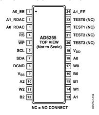
Figure 3. Pin Configuration
