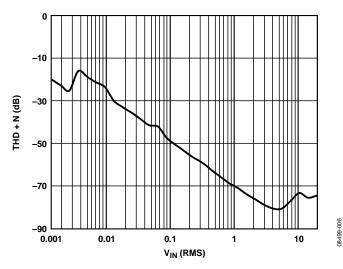
Figure 6. THD + Noise vs. 1 kHz Input Signal Amplitude, 0 dB Gain
