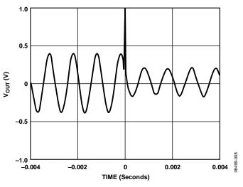
Figure 8. Small Change in Attenuation Showing Glitch Without Glitch Reduction Circuit
