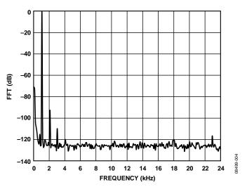
Figure 4. FFT for 1 kHz, 1 V<sub>RMS</sub> Input Signal, 0 dB Gain
