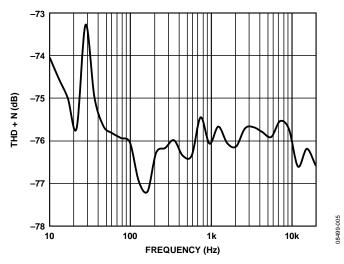
Figure 5. THD + Noise vs. Frequency, 1 V<sub>RMS</sub> Input Signal, 0 dB Gain
