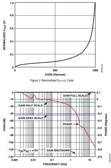
Figure 3. Gain and Phase vs. Frequency for 1 V<sub>RMS</sub> Input Signal
