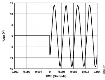
Figure 7. Large Step Change in Attenuation Shows Glitch Without Glitch Reduction Circuit
