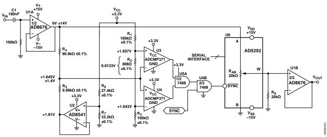
Figure 1. Logarithmic Audio Volume Control with Glitch Reduction (Simplified Schematic: Decoupling and All Connections Not Shown)
