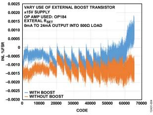
Figure 4. Current Output Mode With/Without Boost Transistor
