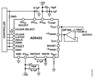
Figure 1. AD5422 Iout and Vout Connected Together
