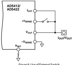
Figure 9. Use of External Switch
