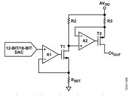
Figure 5. Voltage to Current Conversion Circuitry
