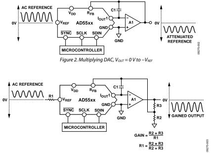
Figure 3. Signal Gain Using Multiplying DACs
