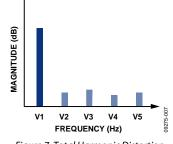
Figure 7. Total Harmonic Distortion
