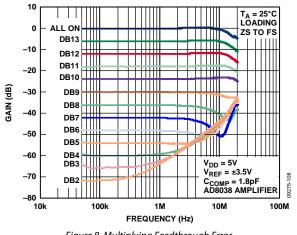
Figure 8. Multiplying Feedthrough Error
