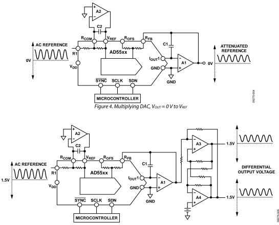
Figure 5. Single-Ended-to-Differential Configuration
