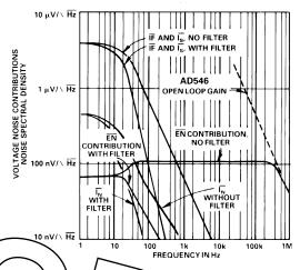
Figure 42. Photodode Preamp Noise Sources' Spectral
