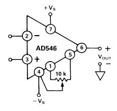
Figure 29. Standard Offset Null Circuit
