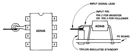
Figure 28. Input Pin to Insulating Standoff
