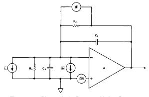
Figure 41. Photodiode Preamp Noise Sources
