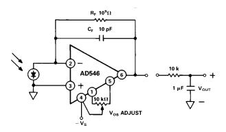
Figure 39. Photodiode Preamp
