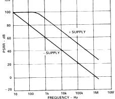
Figure 16. PSRR vs. Frequency
