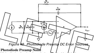
Noise limits the signal resolution obtainable with the preamp. The output voltage noise divided by the feedback resistance is the minimum current signal that can be detected. This minimum detectable current divided by the responsivity of the photodiode represents the lowest light power that can be detected by the preamp.
