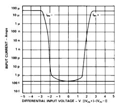
Figure 34. Input Current vs. Differential Input Voltage
