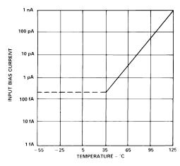
Figure 24. AD546 Input Bias Current vs Ambient Temperature
