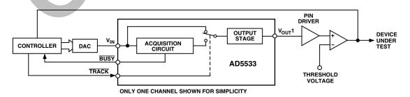
Figure 7. Typical ATE Circuit Using TRACK Input
