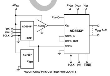
Figure 14. Typical Application Circuit
