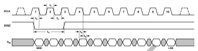
Figure 3. 10-Bit Write (ISHA Mode and Both Readback Modes)
