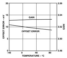
TPC 2. Offset Error and Gain vs. Temperature
