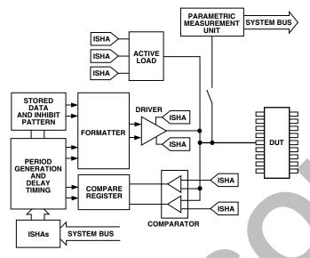
Figure 13. AD5533 in an ATE System
