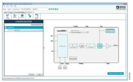
Figure 3. Chip Block Diagram View of the AD5693R
