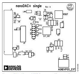
Figure 9. EVAL-AD5693RSDZ Component Placement Drawing
