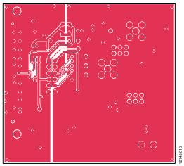
Figure 11. EVAL-AD5693RSDZ Solder Side PCB Drawing
