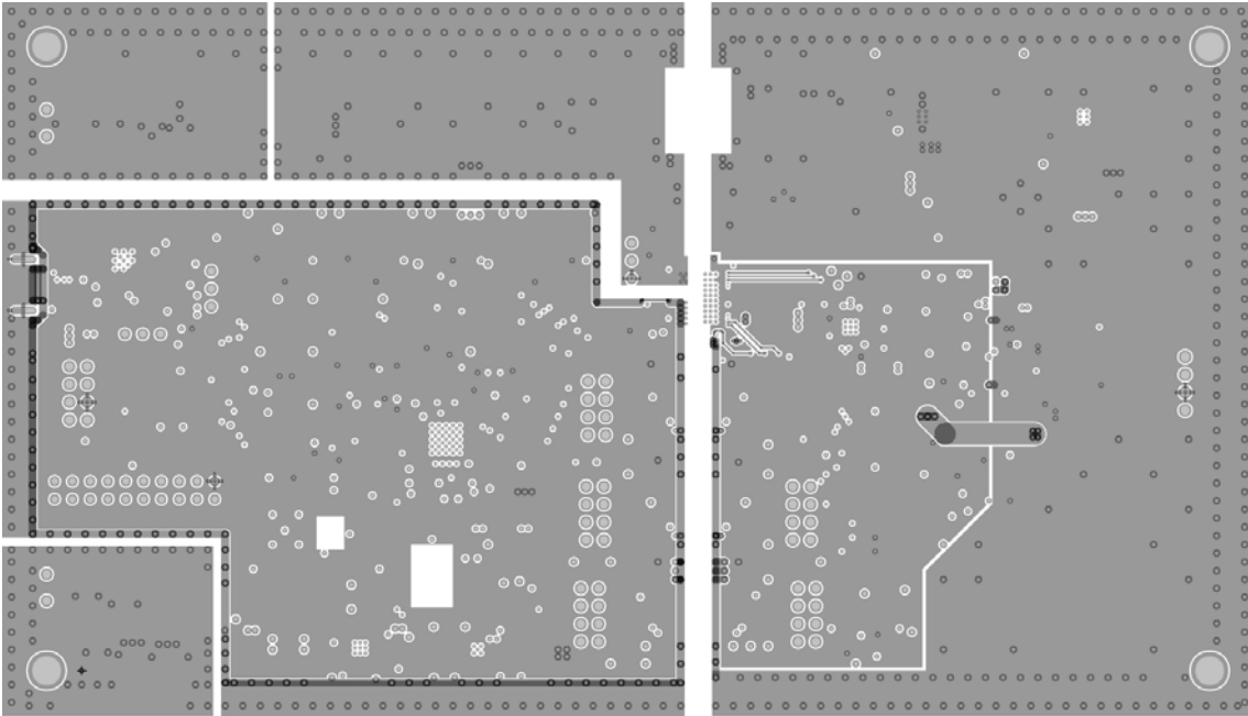
Figure 69. Layer 3, Inner Power Plane
