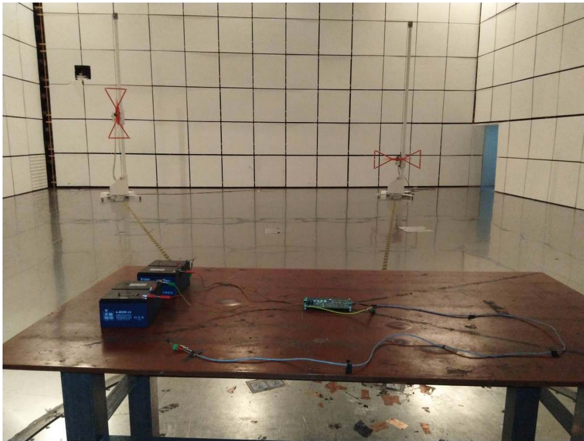
Figure 58. CISPR 11 Radiated Emission Test Setup Photograph
