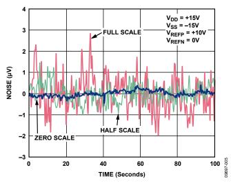
Figure 5. DAC Output Voltage Noise Measured Over 100 Second Period for Full Scale (Red), Half Scale (Green), and Zero Scale (Blue) with Precision Reference Source
