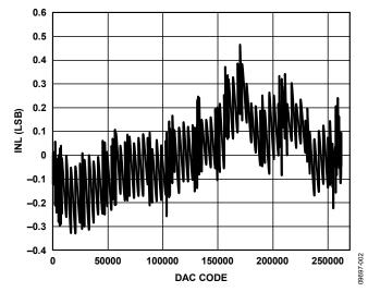
Figure 2. Integral Nonlinearity vs. DAC Code
