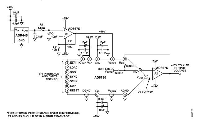
Figure 1. 18-Bit Accurate, +10 V Voltage Source (Simplified Schematic: All Connections and Decoupling Not Shown)
