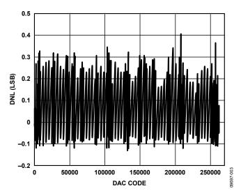
Figure 3. Differential Nonlinearity vs. DAC Code
