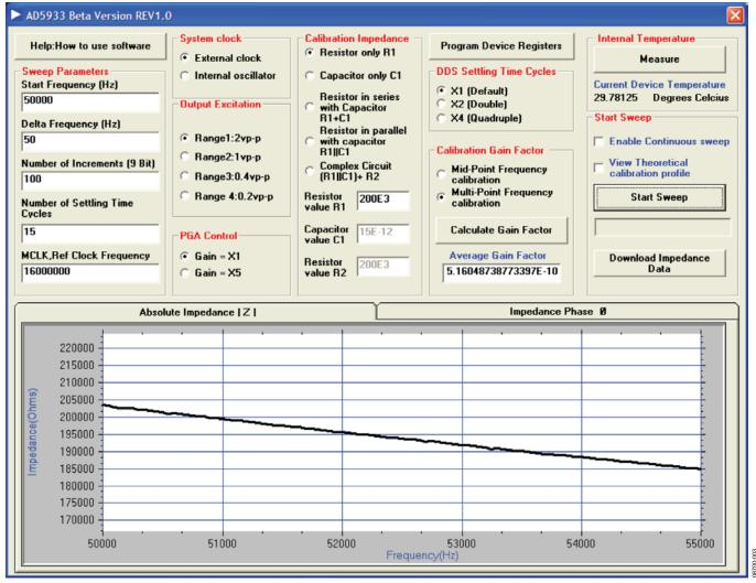
Figure 3. Measuring the Impedance of Capacitor
