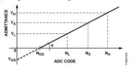
Figure 3. Two Point Calibration for Conductivity Measurement
