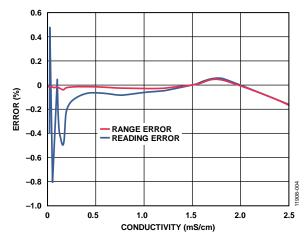
Figure 4. Relative Errors in the Low Range (from 25 μS to 2.5 mS)
