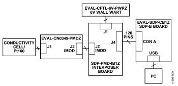
Figure 9. Test Setup Functional Block Diagram
