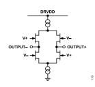
Figure 30. LVDS Outputs (PDOR±, PD[5:0]±, PCLK±)
