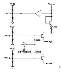
Figure 26. DC Equivalent Analog Input Circuit
