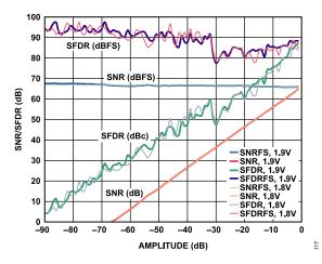
Figure 17. SNR/SFDR vs. Input Amplitude; 500 MSPS, 140.3 MHz
