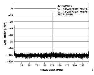
Figure 21. 16k Point Single-Tone FFT; 491.52 MSPS,  $f_{\rm IN1}$  = 121.3 MHz,  $f_{\rm IN2}$  = 124.7 MHz
