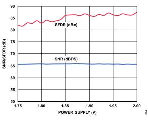
Figure 24. SNR/SFDR vs. Power Supply
