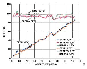
Figure 22. Two-Tone SFDR vs. Input Amplitude; 500 MSPS, 119.2 MHz, 122.5 MHz
