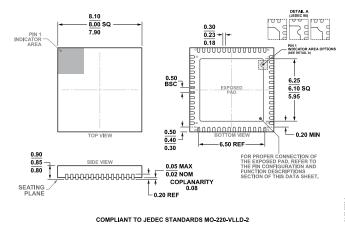
Figure 44. 56-Lead Lead Frame Chip Scale Package [LFCSP] 8 mm × 8 mm Body and 0.85 mm Package Height (CP-56-22) Dimensions shown in millimeters
