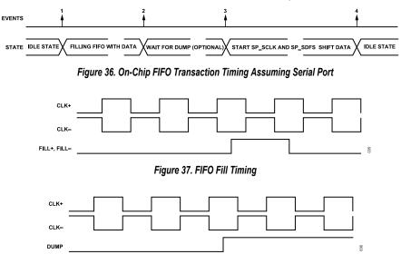
Figure 38. FIFO DUMP Timing
