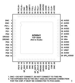
Figure 9. Pin Configuration for Parallel CMOS Mode
