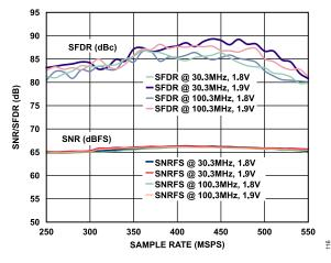
Figure 16. SNR/SFDR vs. Sample Rate and Supply
