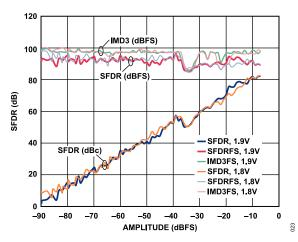
Figure 23. Two-Tone SFDR vs. Input Amplitude; 500 MSPS, 139.3 MHz, 141.3 MHz
