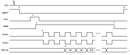
Figure 40. Parallel Mode Transaction Diagram
