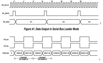
Figure 42. DDR LVDS Output MSB/LSB Interleaving with Decimate by 8
