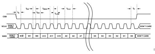
Figure 43. Serial Port Interface Timing Diagram
