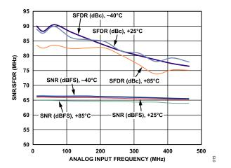
Figure 15. Single-Tone SNR/SFDR vs. Input Frequency (f<sub>IN</sub>) and Temperature; 500 MSPS
