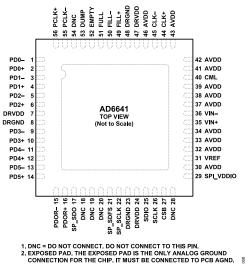
Figure 8. Pin Configuration for DDR LVDS Mode
