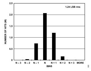
Figure 20. Grounded Input Histogram; 500 MSPS
