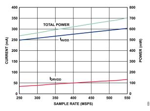
Figure 25. Current and Power vs. Sample Rate
