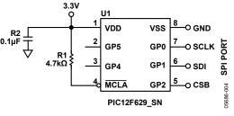
Figure 4. SPI Boot Circuit (Simplified)
