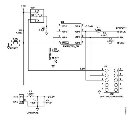
Figure 3. SPI Boot Circuit
