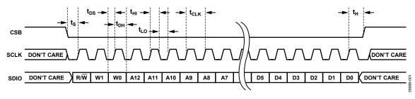
Figure 1. SPI Timing Details
