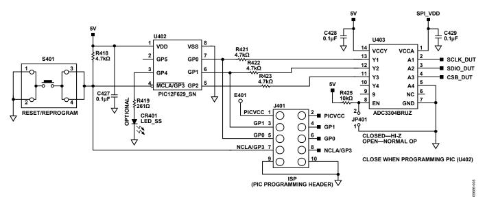
Figure 5. SPI Boot Circuit with Translator
