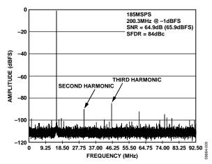
Figure 9. Single Tone FFT,  $f_{IN} = 200.3 \text{ MHz}$
