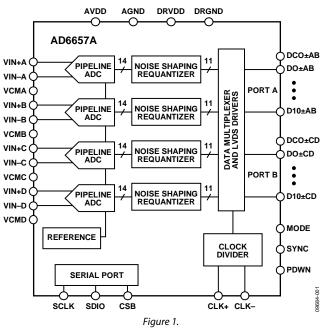
Each ADC output is connected internally to an NSR block. The integrated NSR circuitry allows for improved SNR performance in a smaller frequency band within the Nyquist bandwidth. The device supports two different output modes selectable via the external MODE pin or the serial port interface (SPI).
