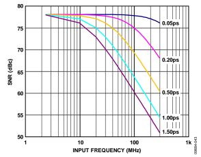
Figure 49. SNR vs. Input Frequency and Jitter
