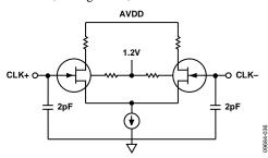
Figure 42. Equivalent Clock Input Circuit
