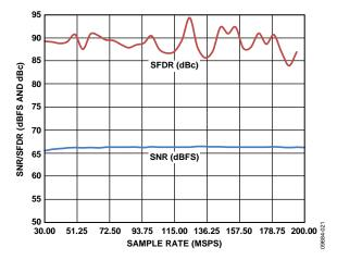
Figure 21. Single Tone SNR/SFDR vs. Sample Rate ( $f_s$ ),  $f_{IN} = 140.3 \text{ MHz}$
