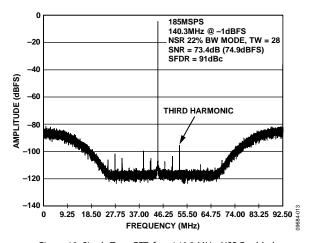
Figure 13. Single Tone FFT,  $f_{\rm IN}$  = 140.3 MHz, NSR Enabled in 22% BW Mode, Tuning Word = 28
