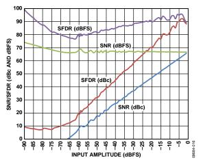
Figure 16. Single Tone SNR/SFDR vs. Input Amplitude ( $A_{IN}$ ),  $f_{IN} = 70.3 \text{ MHz}$
