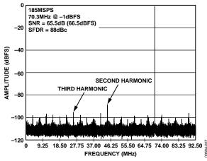
Figure 7. Single Tone FFT,  $f_{IN} = 70.3 \text{ MHz}$
