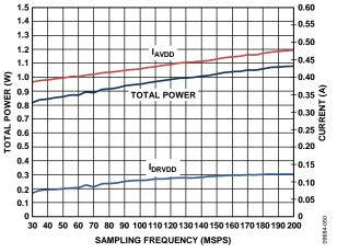
Figure 50. Power and Current vs. Sampling Frequency
