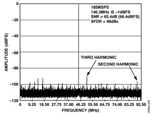
Figure 8. Single Tone FFT,  $f_{IN} = 140.3 \text{ MHz}$
