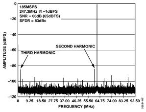
Figure 11. Single Tone FFT,  $f_{IN} = 247.3 \text{ MHz}$
