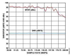
Figure 20. Single Tone SNR/SFDR vs. Sample Rate ( $f_s$ ),  $f_{IN} = 70.3 \text{ MHz}$
