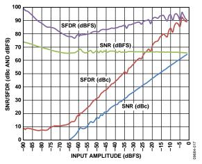
Figure 17. Single Tone SNR/SFDR vs. Input Amplitude ( $A_{IN}$ ),  $f_{IN} = 140.3 \text{ MHz}$
