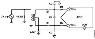
Figure 37. Differential Transformer-Coupled Configuration
