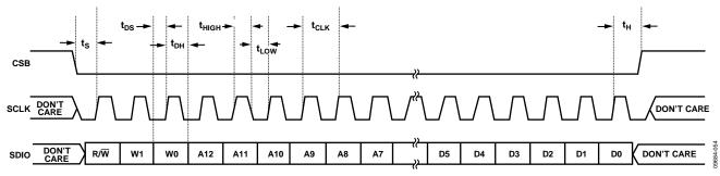
Figure 60. Serial Port Interface Timing Diagram
