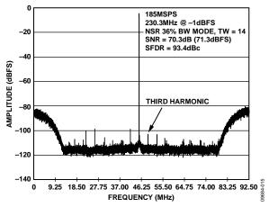
Figure 15. Single Tone FFT, f<sub>IN</sub> = 230.3 MHz, NSR Enabled in 36% BW Mode, Tuning Word = 14
