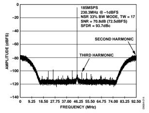
Figure 14. Single Tone FFT,  $f_N = 230.3$  MHz, NSR Enabled in 33% BW Mode, Tuning Word = 17
