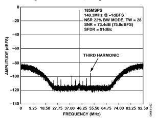
Figure 52. 22% BW Mode, Tuning Word =  $28 (f_s/4 \text{ Tuning})$
