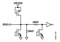
Figure 34. Equivalent SDIO Circuit
