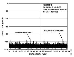
Figure 6. Single Tone FFT,  $f_{IN} = 50.3 \text{ MHz}$
