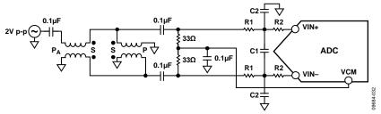
Figure 38. Differential Double Balun Input Configuration
