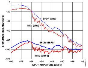
Figure 23. Two Tone SFDR/IMD3 vs. Input Amplitude (A<sub>IN</sub>),  $f_{\rm IN1}=169.1$  MHz and  $f_{\rm IN2}=172.1$  MHz
