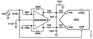
Figure 36. Differential Input Configuration Using the ADA4938-2
