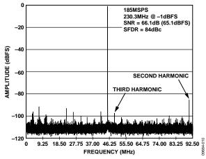
Figure 10. Single Tone FFT,  $f_{IN} = 230.3 \text{ MHz}$
