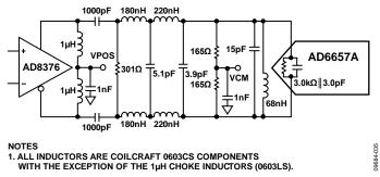
Figure 41. Active Front-End Configuration Using the AD8376
