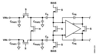
Figure 35. Switched Capacitor Input
