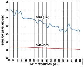
Figure 19. Single Tone SNR/SFDR vs. Input Frequency ( $f_{\rm IN}$ ), 2.0 V p-p Full Scale
