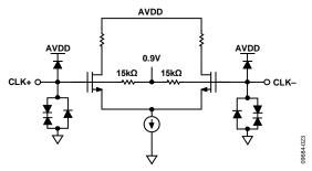
Figure 29. Equivalent Clock Input Circuit
