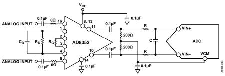
Figure 39. Differential Input Configuration Using the AD8352
