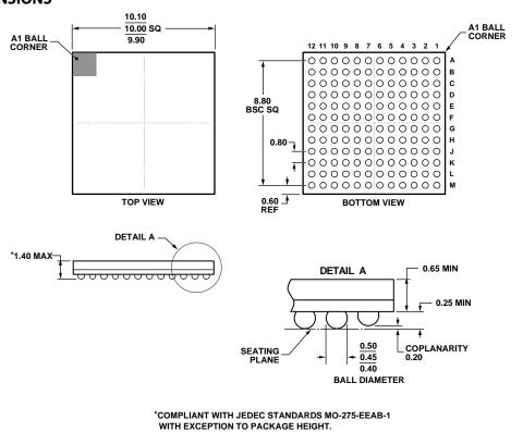
Figure 61. 144-Ball Chip Scale Package Ball Grid Array [CSP\_BGA] (BC-144-1) Dimensions shown in millimeters
