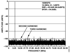
Figure 5. Single Tone FFT,  $f_{IN} = 10.3 MHz$
