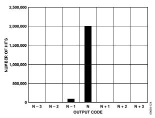
Figure 24. Grounded Input Histogram
