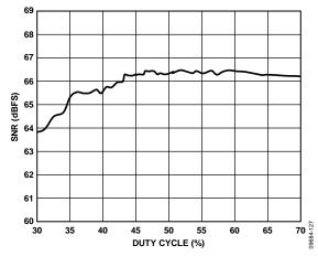
Figure 27. SNR vs. Duty Cycle,  $f_{IN} = 10.3 \text{ MHz}$
