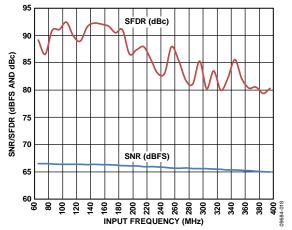
Figure 18. Single Tone SNR/SFDR vs. Input Frequency  $(f_{IN})$ , 1.75 V p-p Full Scale
