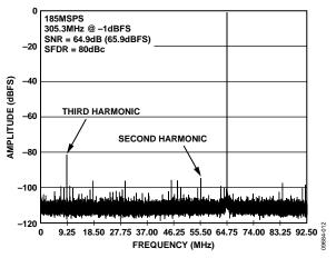
Figure 12. Single Tone FFT,  $f_{IN} = 305.3 \text{ MHz}$
