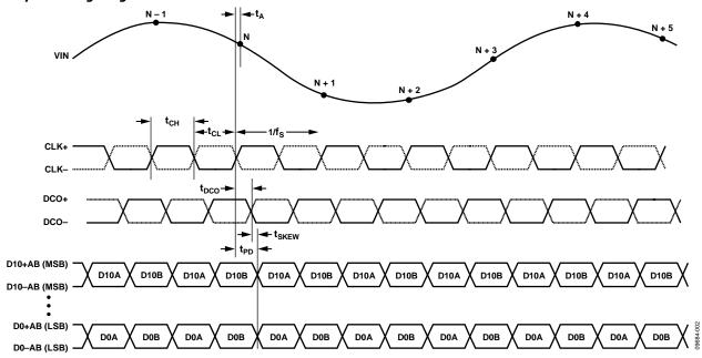
Figure 2. Data Output Timing (Timing for Channel C and Channel D Is Identical to Timing for Channel A and Channel B)
