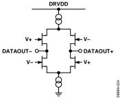
Figure 30. Equivalent LVDS Output Circuit
