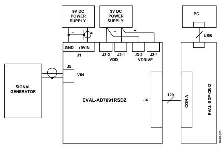
Figure 5. Functional Diagram of Test Setup
