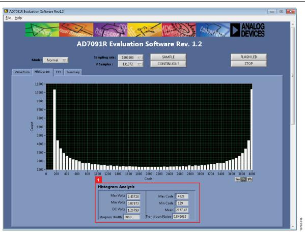
Figure 16. Histogram Capture Tab
