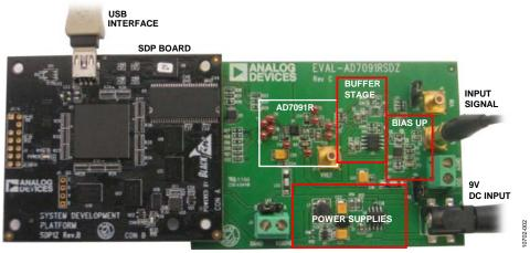
Figure 2. Hardware Configuration—Setting Up the EVAL-AD7091RSDZ
