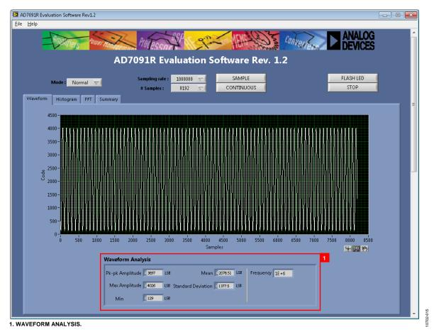
Figure 15. Waveform Capture Tab
