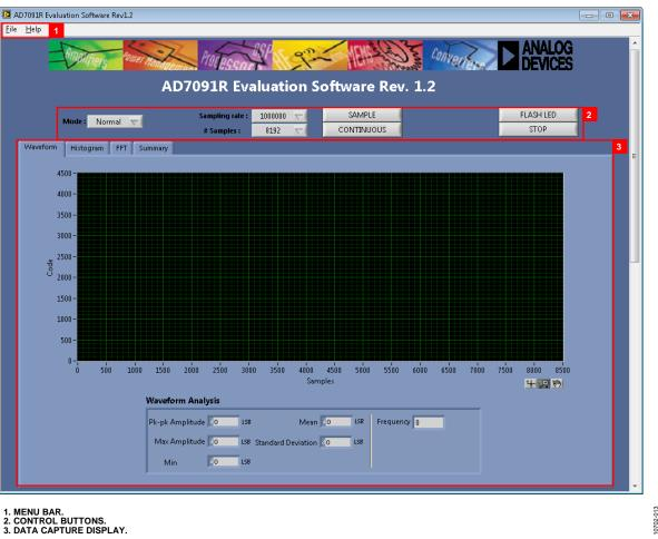
Figure 13. Evaluation Software Main Window
