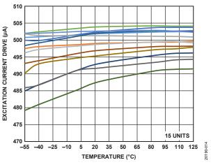
Figure 14. Excitation Current Drift (500  $\mu$ A)
