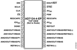
Figure 2. Pin Configuration
