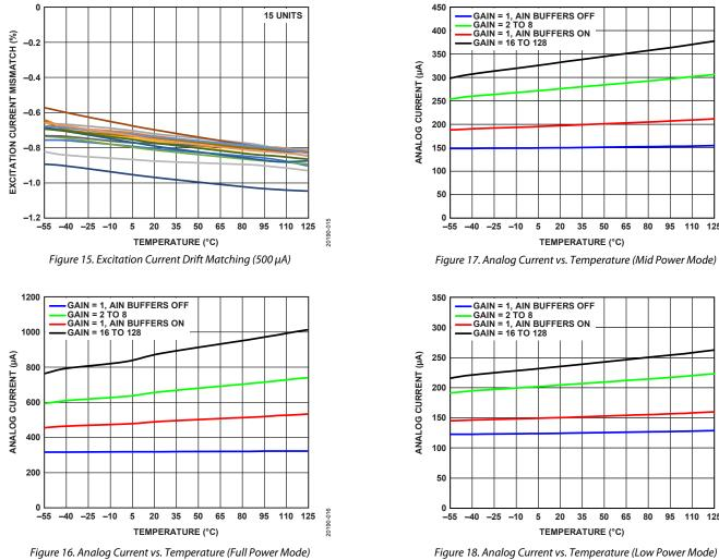
Figure 16. Analog Current vs. Temperature (Full Power Mode)
