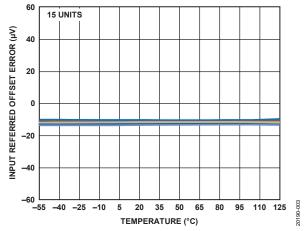
Figure 3. Input Referred Offset Error vs. Temperature (Gain = 8, Full Power Mode)
