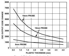
Figure 5. Slider Sensor Activation Response
