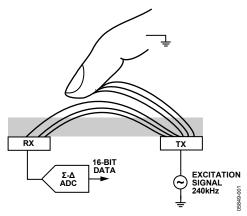
Figure 1. Capacitance Sensing
