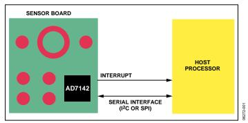
Figure 1. AD7142 System Block Diagram
