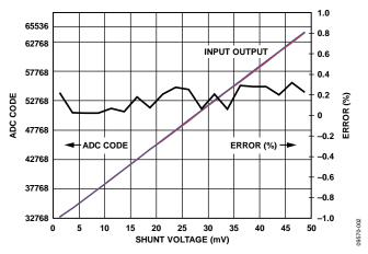
Figure 2. Plot of Output and Error vs. Shunt Voltage
