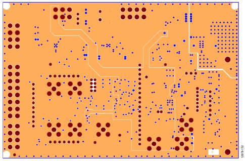
Figure 32. Layer 2 Ground Plane
