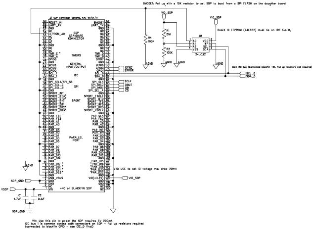
Figure 28. SDP-B Connector Schematic
