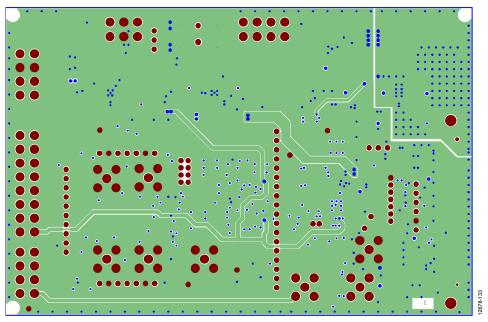
Figure 33. Layer 3 Power/Ground Plane
