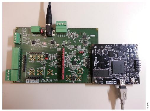
Figure 2. Hardware Configuration, Setting Up the EVAL-AD7172-4SDZ
