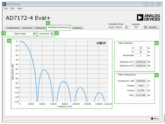
Figure 19. Filter Profiles of the AD7172-4 Evaluation Software
