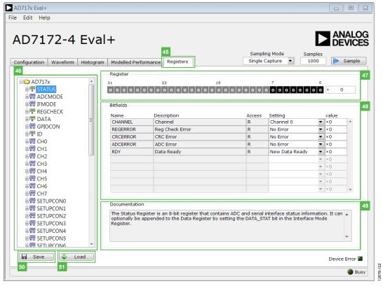
Figure 22. Registers Tab of the AD7172-4 Evaluation Software
