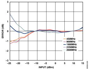
Figure 8. Measured VRMS Linearity Error vs. Input Level, 450 MHz, 900 MHz, 1900 MHz, 2350 MHz, 2600 MHz, Supply +3.3 V
