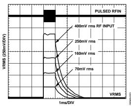
Figure 6. Output Response to Various RF Input Pulse Levels, Supply3 V, 900 MHz Frequency, Square-Domain Filter Open, Output Filter 0.1 μF
