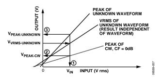
Figure 10. Procedure for Crest Factor Calculation
