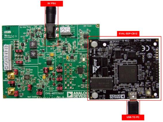
Figure 2. Hardware Configuration—Setting up the EVAL-AD7276SDZ (EVAL-AD7276SDZ on Left and EVAL-SDP-CB1Z on Right)
