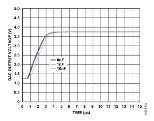
Figure 22. Settling Time for a ¼ to ¾ Output Voltage Step
