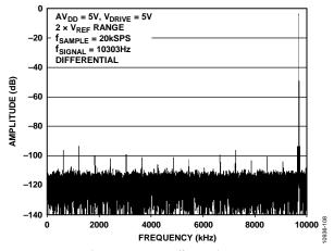
Figure 8. Signal-to-Noise Ratio, Differential Input,  $2 \times V_{REF}$  Range
