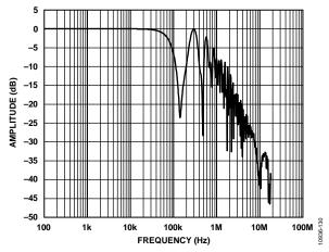
Figure 30. Frequency Response of the High-Side Current Sensor
