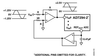
Figure 34. Single-Ended Mode Connection Diagram
