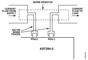
Figure 41. Kelvin Sense Connections (RSx Can Be Either RS1 or RS2)
