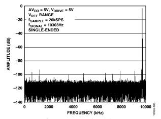
Figure 5. Signal-to-Noise Ratio, Single-Ended Input, VREF Range
