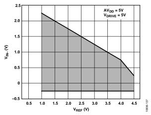
Figure 36. V<sub>IN-</sub> Input Range vs. V<sub>REF</sub> in Pseudo Differential Mode
