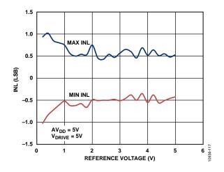
Figure 17. ADC INL vs. Reference Voltage
