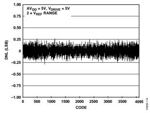
Figure 15. ADC DNL, Differential Input,  $2 \times V_{REF}$  Range
