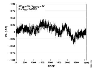
Figure 14. ADC INL, Differential Input, VREF Range
