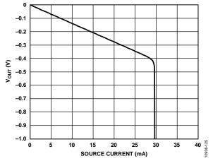
Figure 25. DAC Sourcing Current at Input Code = 0xFFF,  $(V_{OUT} = AV_{DD})$
