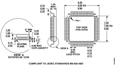
Figure 58. 64-Lead Thin Plastic Quad Flat Package [TQFP] (SU-64-1) Dimensions shown in millimeters
