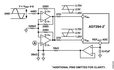
Figure 38. Dual Op Amp Circuit to Convert a Single-Ended Bipolar Signal into a Differential Unipolar Signal Rev. 0 | Page 20 of 44
