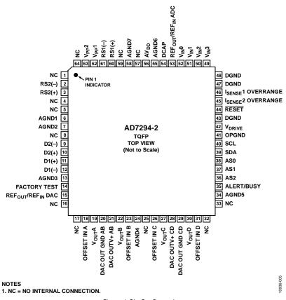
Figure 4. Pin Configuration
