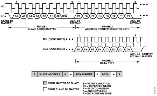
Figure 48. Single Byte Write Sequence
