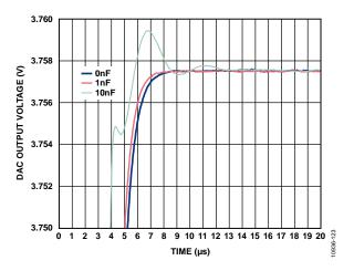
Figure 23. Zoomed-In Settling Time for a ¼ to ¾ Output Voltage Step
