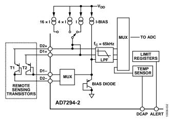
Figure 42. Internal and Remote Temperature Sensors
