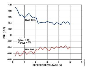
Figure 18. ADC DNL vs. Reference Voltage
