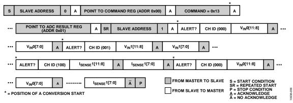
Figure 53. Command Mode Operation
