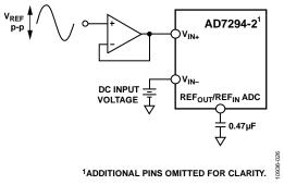
Figure 37. Pseudo Differential Mode Connection Diagram
