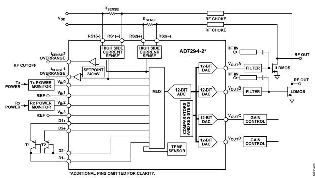
Figure 56. Typical HPA Monitor and Control Application
