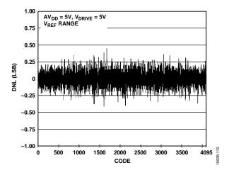
Figure 10. ADC DNL, Single-Ended Input, VREF Range
