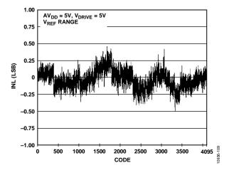
Figure 9. ADC INL, Single-Ended Input, VREF Range
