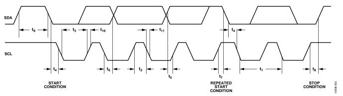
$\textit{Figure 2. } 1^2 \textit{C-Compatible Serial Interface Timing Diagram}$
