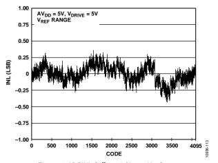
Figure 13. ADC INL, Differential Input,  $V_{REF}$  Range
