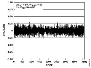
Figure 16. ADC DNL, Differential Input, 2 × V<sub>REF</sub> Range
