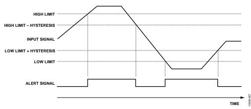
Figure 55. Limit Checking
