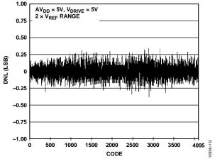
Figure 12. ADC DNL, Single-Ended Input,  $2 \times V_{REF}$  Range
