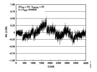
Figure 11. ADC INL, Single-Ended Input,  $2 \times V_{REF}$  Range
