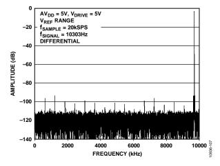
Figure 7. Signal-to-Noise Ratio, Differential Input, VREF Range
