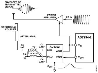
Figure 57. Setpoint Controller Operation
