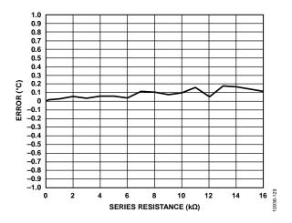
Figure 29. Temperature Error vs. Series Resistance
