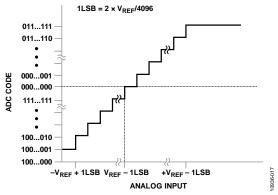
Figure 33. Differential Transfer Characteristics with  $V_{REF} \pm V_{REF}$  Input Range
