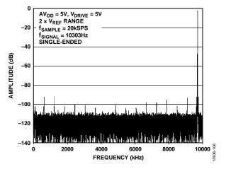
Figure 6. Signal-to-Noise Ratio, Single-Ended Input,  $2 \times V_{REF}$  Range
