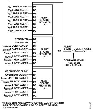
Figure 54. Alert Status Register Structure
