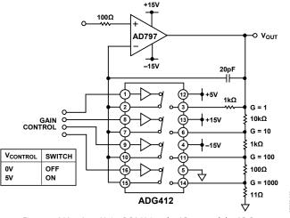
Figure 9. A Very Low Noise PGA Using the AD797 and the ADG412
