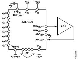
Figure 8. Programmable Gain Amplifier Between MUXout and ADCIN Configuration for AD7329
