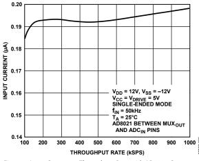
Figure 5. Input Current vs. Throughput Rate with AD8021 Connected Between  $MUX_{OUT}$  and ADC  $_{\rm IN}$  Pins
