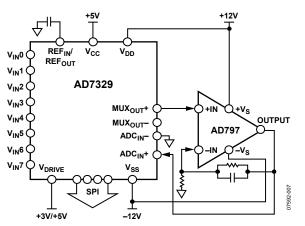
Figure 7. Gain Stage Between MUXout and ADCIN Configuration for AD7329
