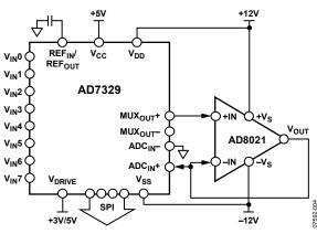
Figure 4. Buffer Between MUXout and ADCIN Configuration for AD7329
