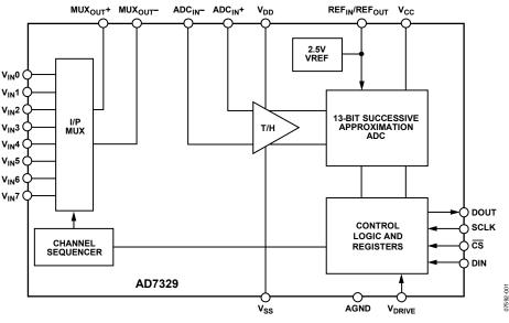
Figure 1. AD7329 Functional Block Diagram
