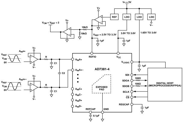
NOTES 1. V- IS THE EXTERNAL SUPPLY VOLTAGE (-2.5 V) FOR THE DRIVER AMPLIFIER. 2. PLACE DECOUPLING CAPACITORS CLOSE TO (IDEALLY, RIGHT UP AGAINST) THE DEVICE SUPPLY PINS AND REFERENCE PIN.
