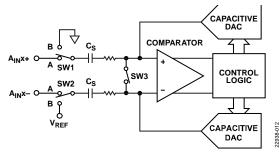
Figure 27. ADC Acquisition Phase
