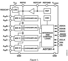
The AD7381-4 is available in a 24-lead lead frame chip scale package (LFCSP) with operation specified from  $-40^{\circ}$ C to  $+125^{\circ}$ C.
