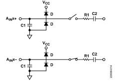
Figure 29. Equivalent Analog Input Circuit, Conversion Phase—Switches Open, Track Phase—Switches Closed
