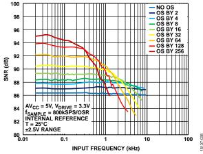
Figure 17. SNR vs. Input Frequency for Different OSR Values, ±2.5 V Range, Internal OS Clock
