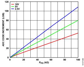
Figure 61. Open Circuit Code Error Increment, Dependent of R<sub>PD</sub>
