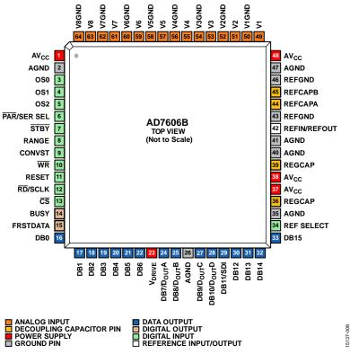
Figure 8. Pin Configuration
