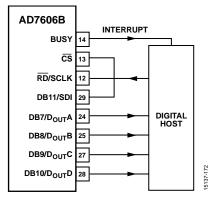
Figure 70. AD7606B Interface Diagram—One AD7606B Using the Serial Interface with Four Dourx Lines
