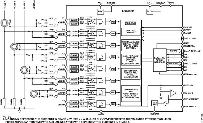
NOTES 1. IXP AND IXN REPRESENT THE CURRENTS IN PHASE X, WHERE X = A, B, C, OR N. VXN/VXP REPRESENT THE VOLTAGES AT THESE TWO LINES. FOR EXAMPLE, IAP (POSITIVE PATH) AND IAN (NEGATIVE PATH) REPRESENT THE CURRENTS IN PHASE A.
