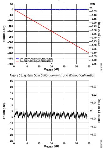
Figure 59. System Error with Gain Calibration Enabled
