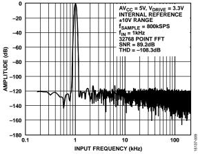
Figure 9. Fast Fourier Transform (FFT), ±10 V Range
