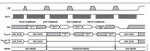
Figure 74. AD7606B Register Mode
