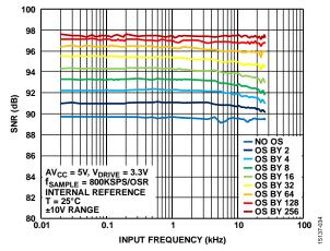
Figure 18. SNR vs. Input Frequency for Different OSR Values, ±10 V Range, External OS Clock
