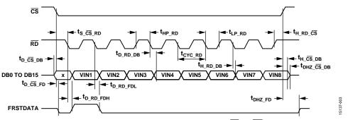
Figure 3. Parallel Mode Read Timing Diagram, Separate  $\overline{\text{CS}}$  and  $\overline{\text{RD}}$  Pulses
