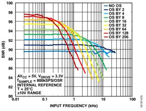
Figure 15. SNR vs. Input Frequency for Different OSR Values, ±10 V Range, Internal OS Clock
