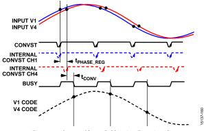
Figure 56. System Phase Calibration Functionality
