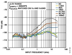
Figure 26. THD vs. Input Frequency for Various Source Impedances, ±2.5 V Range
