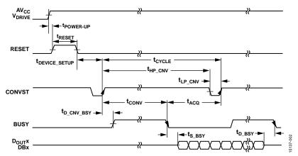
Figure 2. Universal Timing Diagram
