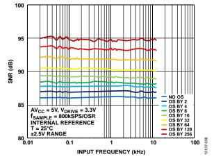
Figure 20. SNR vs. Input Frequency for Different OSR Values, ±2.5 V Range, External OS Clock
