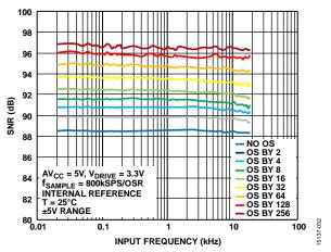
Figure 19. SNR vs. Input Frequency for Different OSR Values, ±5 V Range, External OS Clock
