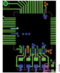
Figure 89. Top Layer Decoupling REFIN/REFOUT, REFCAPA, REFCAPB, and REGCAP Pins
