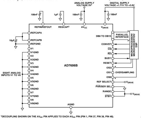
$^1\text{DECOUPLING}$  SHOWN ON THE AV\_{CC} PIN APPLIES TO EACH AV\_{CC} PIN (PIN 1, PIN 37, PIN 38, PIN 48). DECOUPLING CAPACITOR CAN BE SHARED BETWEEN AV\_{CC} PIN 37 AND PIN 38.  $^2\text{DECOUPLING}$  SHOWN ON THE REGCAP PIN APPLIES TO EACH REGCAP PIN (PIN 36, PIN 39).
