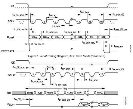
Figure 7. Serial Interface Timing Diagram, Register Map Read/Write Operations
