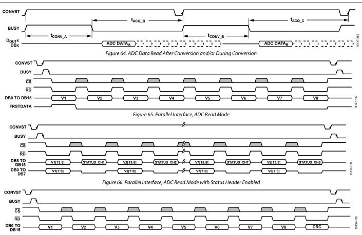
Figure 67. Parallel Interface, ADC Read Mode with CRC Enabled
