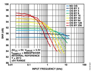
Figure 16. SNR vs. Input Frequency for Different OSR Values, ±5 V Range, Internal OS Clock
