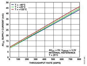
Figure 40. AV<sub>CC</sub> Supply Current vs. Throughput Rate
