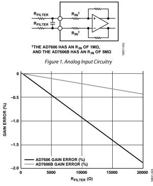
Figure 2. Gain Error Introduced by the Input Series Resistor (R<sub>FILTER</sub>)
