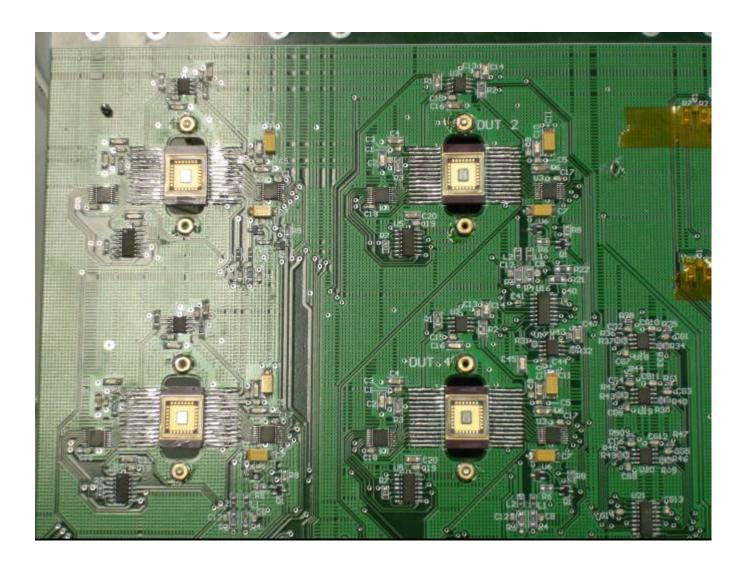
Figure 3.1. Single event test board that was mounted on the test stage at Berkeley. The board has four unitsunder-test (labeled as DUTs 1, 2, 3 and 4) mounted simultaneously to minimize vacuum breaks during testing. There is also a heater plate mounted to the backside of the board to provide the elevated temperature required for this testing.
