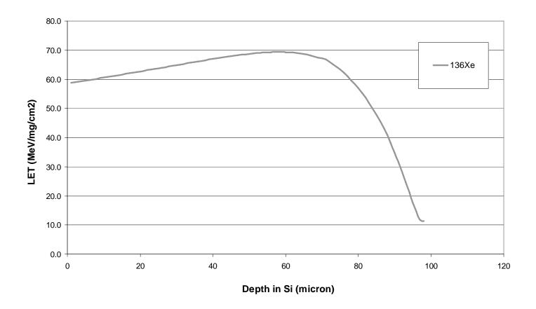
Figure 3.1. Range of the 10MeV/n Xe beam into silicon. The range to the Bragg Peak for Xe (the shortest range ion used) is approximately  $60\mu$ m while the surface LET is approximately 58MeV-cm2/mg.
