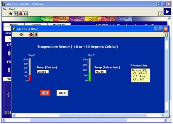
Figure 5. AD7714-3 Evaluation Software Temperature Demo Window
