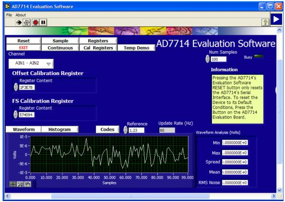
Figure 4. AD7714-3 Evaluation Software Cal Registers Window
