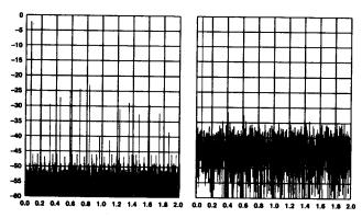
The right-hand figure shows the A/D output after a dither signal that is 4 dB above the quantization noise floor is added to the input. In this case the quantization noise depends on the magnitude of the dither signal at the instant when a sample is taken. Since the value of the dither doesn't depend on the input signal, the quantization noise becomes uncorrelated to the input and the harmonics in the A/D spectrum are eliminated, but at the cost of an overall increase in the noise floor.
