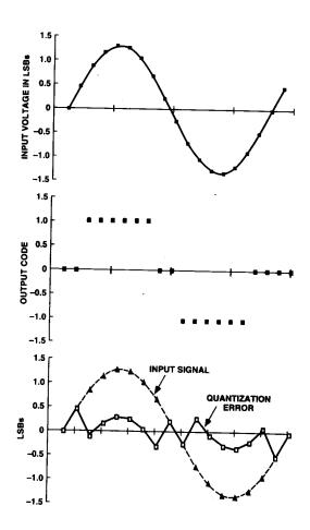
Another way to look at this phenomenon is to consider the case when the (sinusoidal) input signal is only around 1 LSB in size and the digital output resembles a square wave. Square waves are rich in harmonics! The harmonics, or noise modulation products, are very objectionable in many converter applications, especially audio.
