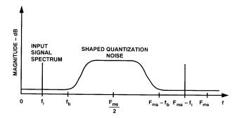
As shown, the spectral "sticks" (single frequencies) at  $f_i$  and  $F_{ms}$ – $f_i$  correspond to an input signal, while the shaded area shows how the quantization noise has been pushed (shaped) beyond the bandwidth of interest,  $f_h$ .
