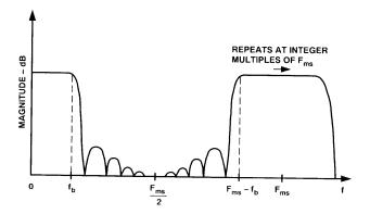
Thus it is the input noise energy in these bands  $[kF_{ms}\pm f_b]$  that must be removed by the antialiasing filter before the input signal is sampled by the converter.
