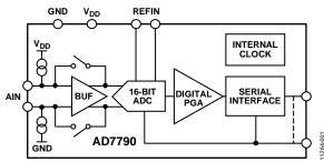
Figure 1. Functional Block Diagram
