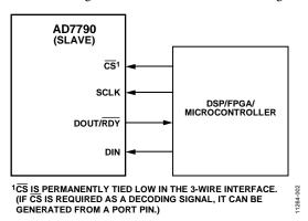
Figure 2. AD7790 Data Interface, 4-Wire SPI
