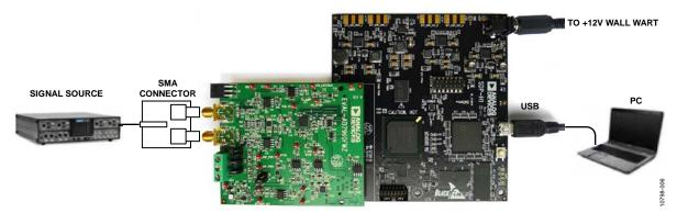
Figure 6. EVAL-AD7960FMCZ Board Connected to EVAL-SDP-CH1Z Board
