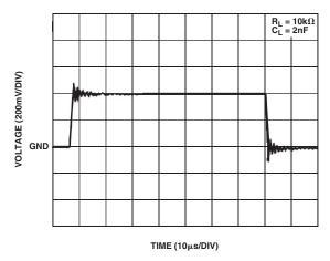
Figure 7. Capacitive Load Drive Without Resistor
