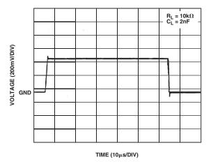
Figure 8. Capacitive Load Drive with Resistor
