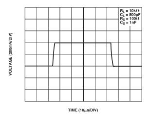
Figure 11. Capacitive Load Drive with the Snubber
