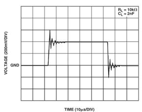
Figure 10. Capacitive Load Drive Without Snubber
