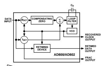
During the process of acquisition the frequency detector provides a Frequency Acquisition (FRAC) signal which indicates that the device has not yet locked onto the input data. This signal is a series of pulses which occur at the points of cycle slip between the input data and the synthesized clock signal. Once the circuit has acquired frequency lock no pulses occur at the FRAC output.
