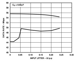
Figure 13. AD800-52 Acquisition Range vs. Input Jitter
