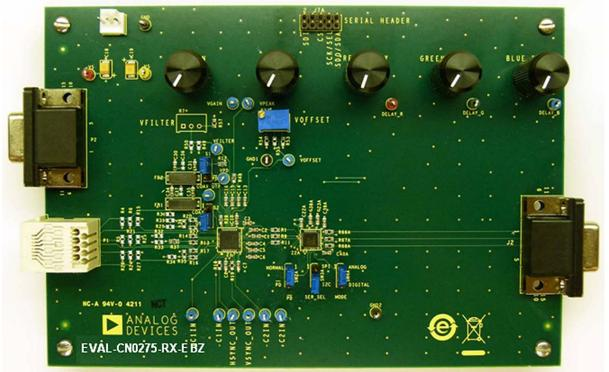
*Figure 10. EVAL-CN0275-RX-EBZ Receiver Evaluation Board*
