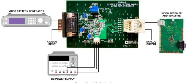
Figure 2. Typical Evaluation Setup
