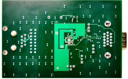
Figure 5. AD8147-EVALZ/AD8148-EVALZ Evaluation Board, Rear Side
