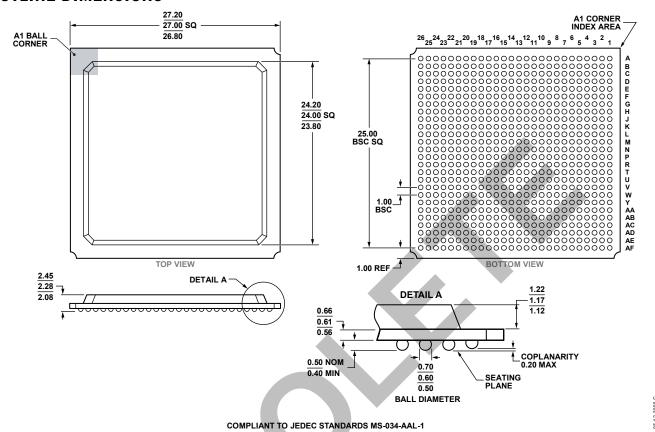
Figure 53. 676-Ball Plastic Ball Grid Array [PBGA] (B-676) Dimensions shown in millimeters
