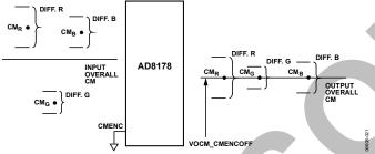
Figure 46. AD8178 in a Middle of Cat-5 Run Application, CM Encoding Off (Note that in this application, the H and V outputs, though asserted, are not used.)
