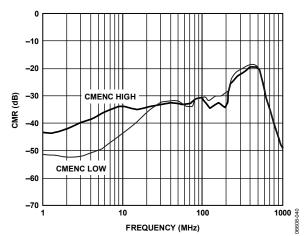
Figure 31. Common-Mode Rejection
