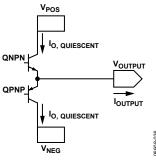
Figure 51. Simplified Output Stage
