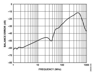
Figure 37. Output Balance Error
