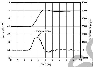
Figure 27. Large Signal Rising Edge Slew Rate
