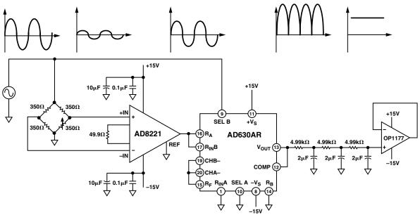
Figure 1. Using an AC Signal to Excite the Bridge
