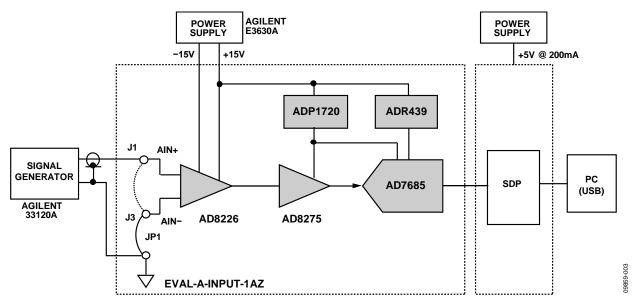
Figure 3. Functional Block Diagram of Test Setup
