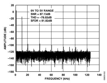
Figure 2. FFT Results for 10 kHz Input Signal 14 dB Below Full-Scale, 250 kSPS Sampling Rate
