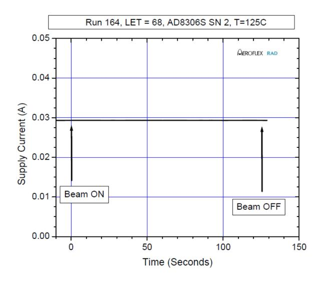
Figure 5.3. Input supply current versus time/fluence for the AD8306 5 MHz–400 MHz 100 dB High Precision Limiting-Logarithmic Amplifier (run 164). See Table 4.1 for the details of the test conditions.
