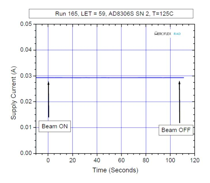
Figure 5.4. Input supply current versus time/fluence for the AD8306 5 MHz–400 MHz 100 dB High Precision Limiting-Logarithmic Amplifier (run 165). See Table 4.1 for the details of the test conditions.
