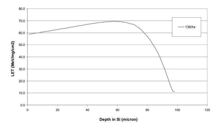
Figure 3.2. Range of the 10MeV/n Xe beam into silicon. The range to the Bragg Peak for Xe (the shortest range ion used) is approximately 60µm while the surface LET is approximately 58MeV-cm2/mg.
