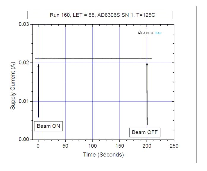
Figure 5.1. Input supply current versus time/fluence for the AD8306 5 MHz–400 MHz 100 dB High Precision Limiting-Logarithmic Amplifier (run 160). See Table 4.1 for the details of the test conditions.
