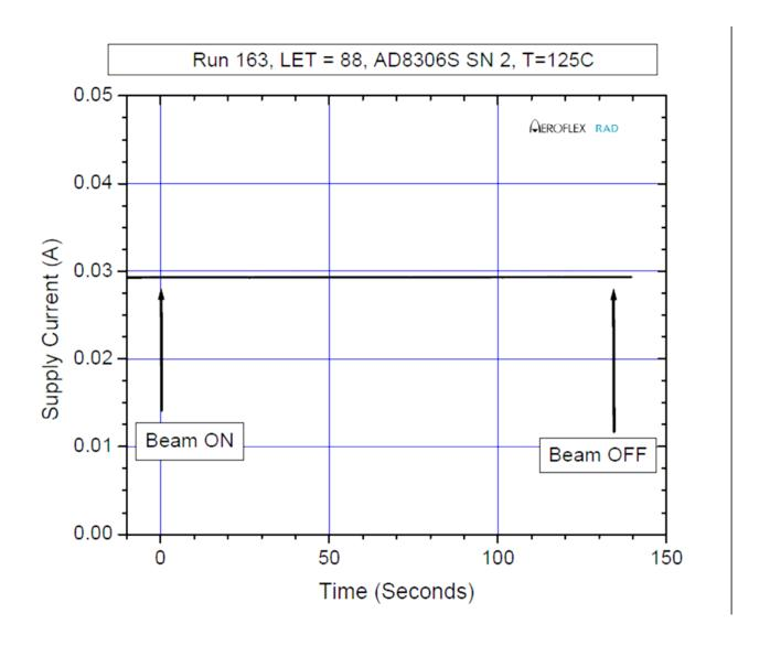
Figure 5.2. Input supply current versus time/fluence for the AD8306 5 MHz–400 MHz 100 dB High Precision Limiting-Logarithmic Amplifier (run 163). See Table 4.1 for the details of the test conditions.
