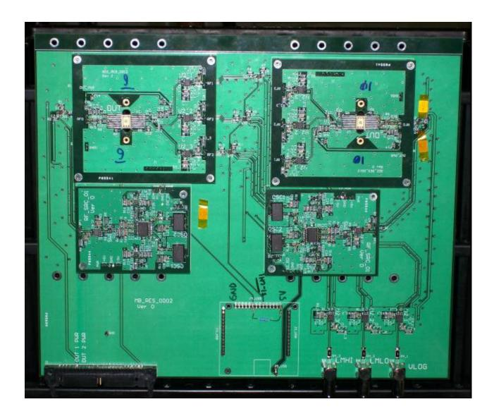
Figure 3.1. Single event test board prepared for mounting on the test stage at Berkeley. The board has two units-under-test mounted simultaneously to minimize vacuum breaks during testing. There is also a heater plate mounted to the backside of the board to provide the elevated temperature required for this testing.
