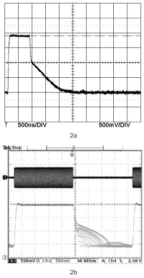
Figure 2. Tails at the output of a log amp in response to RF bursts.
