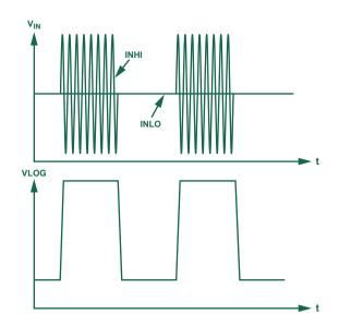
Figure 5. Ideal signals at INHI and INLO when using circuit shown in Figure 4b.
