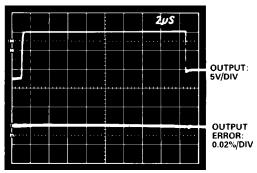
Figure 24. AD840 Settling Demonstrating No Settling Tails
