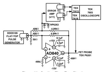
Figure 23. Settling Time Test Circuit
