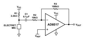
Figure 4. A Microphone Preamplifier
