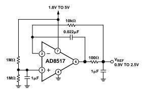
Figure 3. A Micropower Reference Voltage Generator
