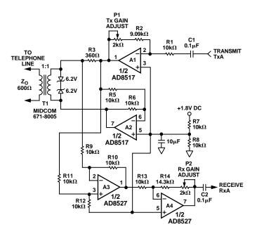
Figure 5. Single-Supply Direct Access Arrangement for Modems
