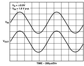
Figure 1. Rail-to-Rail Input Output
