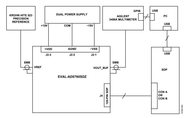
Figure 6. Functional Block Diagram of Test Setup
