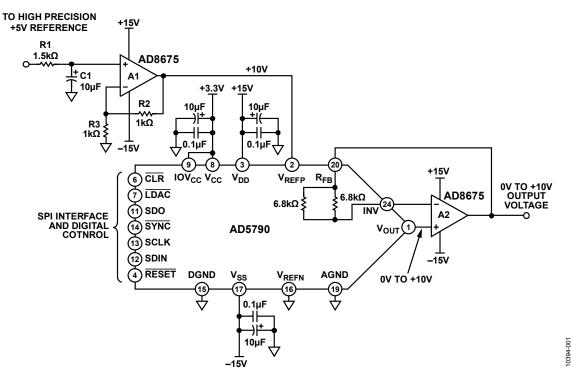
Figure 1. 20-Bit Accurate, 0 V to +10 V Voltage Source (Simplified Schematic: All Connections and Decoupling Not Shown)
